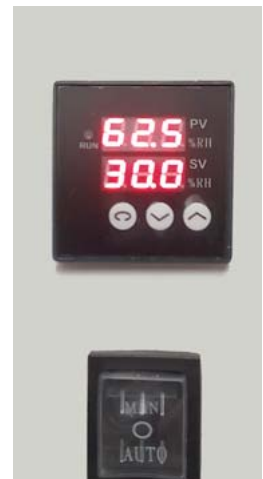
Desiccant dehumidifier control panel
